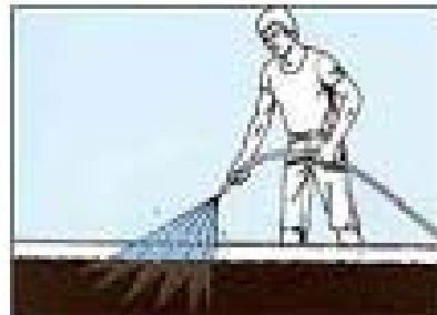
Sub-grade should be damp, but not muddy, Saturate beforehand then sprinkle again just before concrete is placed.
